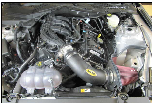
19. Double check your work. Make sure all clamps, hoses, bolts, and screws are tight. Double check the hood clearance. Reconnect the negative battery cable and reinstall the cover.
