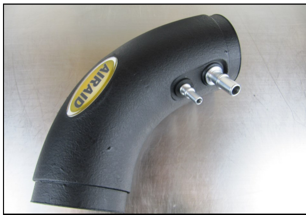
5. Install the Grommets and Aluminum Fittings into the Airaid Intake Tube. Apply the Airaid Bubble Decal onto the Intake Tube as shown.
