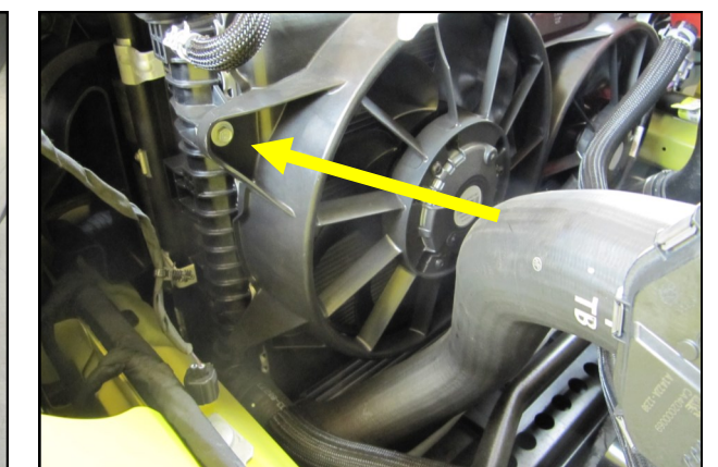
9. Remove the drivers side fan shroud bolt and set it aside.
